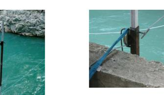
River water velocity at a riverbed cross section (0.5 x0.5 m grid, in ~ 30x5 = 150 points). Measurements for each (at least 3) water level  $\Rightarrow$  river discharge as a function of water level.
