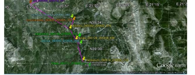
4 double and one single water quality monitoring station are foreseen in combination of eight repeater nodes. In addition a river flow online measurement station are foreseen. 4 single water quality monitoring station are foreseen in combination of three repeater nodes. Two of them were foreseen to interconnect via the Albanian education school network.
